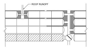
Figure 9 - Perpendicular Inlet
