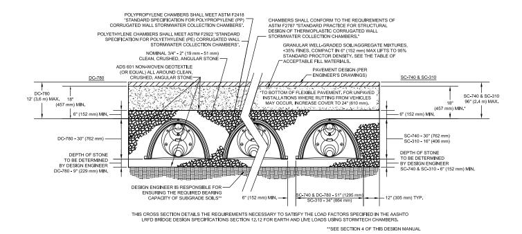
Figure 17 - Inlet and Outlet Detail - StormTech Non-Isolator Row (not to scale)
