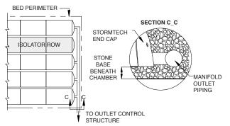
Figure 13 - Combination Outlet SECTION A\_A OUTLET NUMBER AND SIZE OF UNDER- - DRAINS PER ENGINEER DESIGN STORMTECH CHAMBER CONTROL STRUCTURE BED PERIMETER FOUNDATION STONE BENEATH CHAMBER ADS 601 NON-WOVEN GEOTEXTILE (OR EQUAL) SECTION B B STORMTECH END CAP PERFORATED UNDERDRAIN PIPE FOUNDATION STONE | BENEATH ! CHAMBER ADS 601 NON-WOVEN GEOTEXTILE OR EQUAL STONE BEDDING OUTLET CONTROL STRUCTURE PER ENIGNEER'S DESIGN
