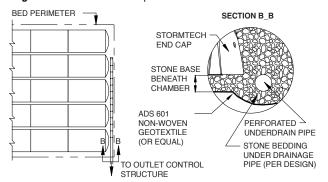
Figure 12 - Outlet Manifold
