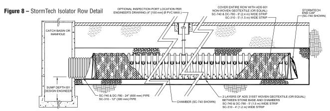
**Note:** For many applications, the non-woven geotextile over the DC-780 Isolator Row chambers can be eliminated or substituted with the AASHTO Class 1 woven geotextile. Contact your StormTech representative for assistance.
