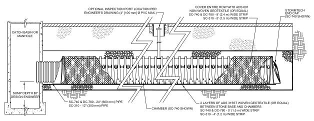
**Note:** For many applications, the non-woven geotextile over the DC-780 Isolator Row chambers can be eliminated or substituted with the AASHTO Class 1 woven geotextile. Contact your StormTech representative for assistance.
