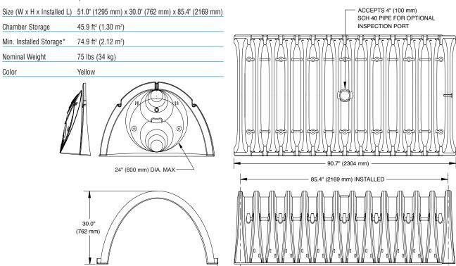
Figure 2 – StormTech SC-310 Chamber (not to scale)
