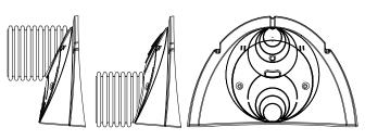
SC-740/DC-780 CHAMBER FABRICATED END CAP (TOP AND BOTTOM FEED) PIPES SIZES RANGE FROM 6" (152 mm) TO 24" (600 mm) (INVERTS VARY WITH PIPE SIZE)
